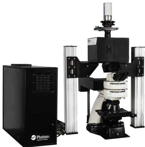
Upright configuration coupled with a CCD camera
